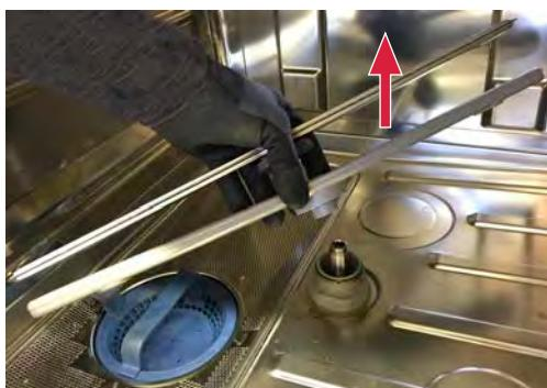
Fit the nozzle insert on the axis instead of the lower arms.
