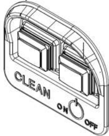
Power Switch Panel
